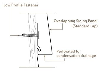
Fasten Panel to Wood with #10-9 Low Profile Wood Screw Install one screw every 24" within pre-punched slots
