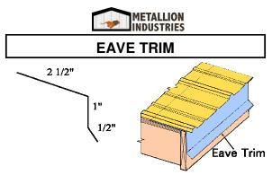
Install the eave trim using low profile screws or nails before installing the panels. For 2/12 roof pitch or less, apply a bead of Clear seal on top of the trim, below the line of screws. You may also use solid foam closure under the panel on top of the Eave Trim to stop rain, snow, etc. from blowing in underneath the panel.
