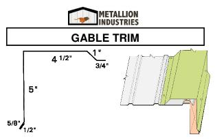
The Gable trim is installed on top of the panel over the rib before the Ridge cap is installed. It is fastened to the fascia board approximately every 24" with 1/4" hex head screws.
