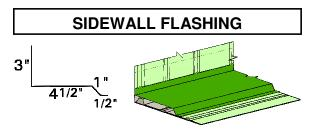
Sidewall flashing is applied when the side of the roof panel runs along an adjacent wall. For the most weather-tight application, the 3" upper leg needs to go behind your wall siding. If that is not an option, see the instructions listed above under Endwall Flashing.
