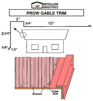
This gable trim is designed for use on a prow-type roof where the ridge is wider than the eave. It is applied the same way as W-Valley. It is basically half of a valley.
