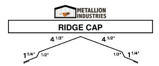
The Ridge cap is used to seal the point at which two upward slopes meet. This can be both along the ridge of the roof as well as a covering for a hip. Install the roof panels by lining them up with the eaves. After the Gable trim is installed, fasten the Ridge cap at every rib of each panel with 3/4" stitch screws.
