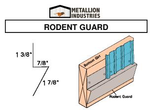
Rodent Guard seals off the bottoms of panels at the floor level, and helps to prevent the entrance of rodents and insects. It also serves well as a base for the setting of panels.
