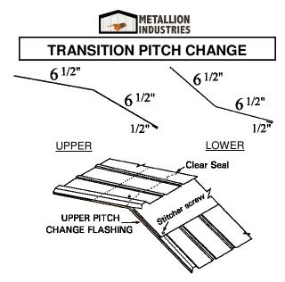
Install panels on the lower pitch first. Under the Pitch Change, you may want to install solid foam closure to stop rain, snow, fir needles, etc. from blowing up under the flashing.
