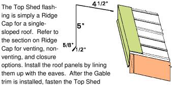
flashing at every rib of each panel with 3/4" stitch screws. You may also fasten through the face of the Top Shed flashing into the fascia or the wall siding.
