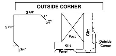
The Outside Corner straddles the ribs of the panels where they meet at the corner of the building. The Inside Corner has similar dimensions but with a reverse middle bend.
