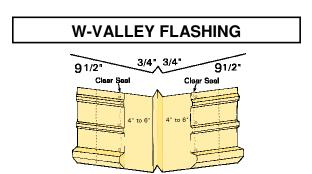
Install W-valley flashing with low profile screws. Cut the panels at the angle of the valley. For 2/12 roof pitch or less, apply a bead of Clear seal on top of the W-valley, below the line of screws.
