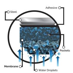
Dripstop is an optional condensation control coating that can be applied to our **Magna Rib** and **PBR** panel profiles at the time of manufacturing.
