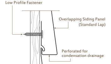
Fasten Panel to Wood with #10-9 Low Profile Wood Screw Install one screw every 24" within pre-punched slots
