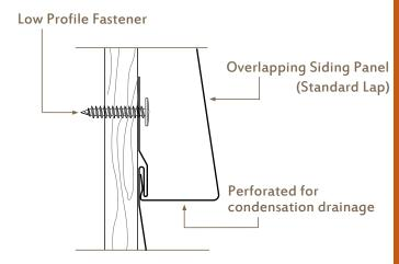
Fasten Panel to Wood with #10-9 Low Profile Wood Screw Install one screw every 24" within pre-punched slots
