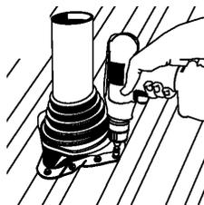
Note: If pipe has a seam, apply sealant where flashing crosses the seam. Apply sealant on upper edge of flashing wherever it is not tight to the roof.
